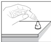
Hold the meter to move the absorbent hole of the test strip to touch the drop. Once the confirmation window fills completely, the meter will begin counting down.
