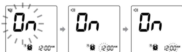
At the time your alarm is set, the meter will beep and automatically turn on. You can press **M** to silence the alarm and insert a test strip to begin testing. If you do not press **M**, the meter will beep for 2 minutes then switch off. If you do not want to test at this time, press **M** to switch off the meter.
