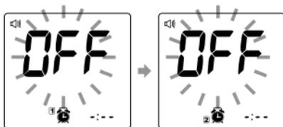
If you do not want to set an alarm, press SET to skip this step. If you want to turn off an alarm, find the alarm number by pressing SET in the setting mode, press
