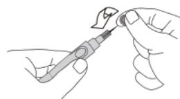
Replace the cap by aligning the arrow on the cap with the release button.
