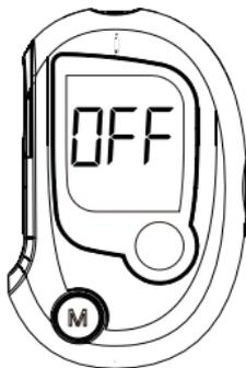
4. If no button is pressed within 2 minutes, the meter will show “OFF” and turn off automatically.
