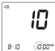
With the minute flashing, press **M** to select the correct minute. Press SET.
